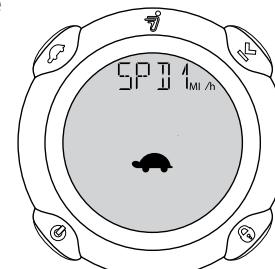
Pressing the Security button (🔒) will display the next available speed. The Beginner Setting speed limit options range from 4.0 mph to 8.0 mph in increments of 0.5 mph.
